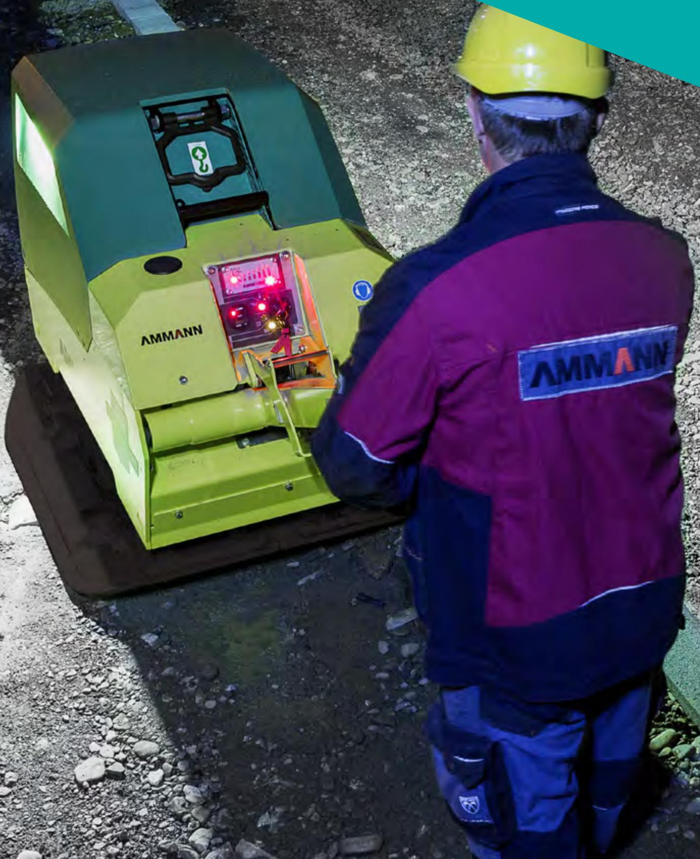
“ With the remote control, the APH 1000 TC allows operation from a secure spot – no danger, no hand-arm vibrations to the operator.”
